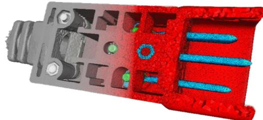
Use the **Volume Meshing Module** to create accurate and high-quality tetrahedral volume meshes from your CT scans which you can then use for mechanical, fluid, thermal, electrical, and other FEM simulations.
